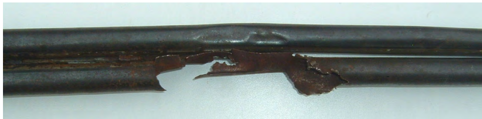
Figure 3-13 – Barrel blocked by mud
