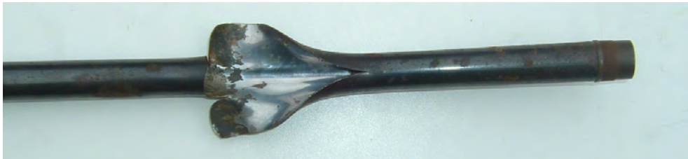
Figure 3-12 – Barrel blocked by a wad
