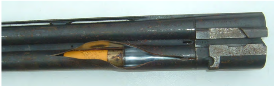
Figure 3-11 – A 20 bore cartridge in a 12 bore barrel
